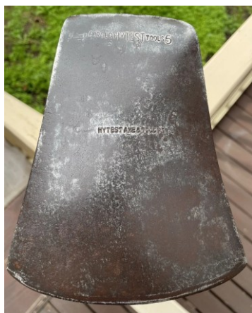
A late 1940s / early 1950s round poll 5lb Hytest Forged Tools work axe with a double stamp on one side. Probably an early version of the Hytest 'Green' work axe.
