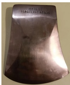
A late 1940s / early 1950s round poll 5lb Hytest Forged Tools work axe with a double stamp on one side. Probably an early version of the Hytest 'Green' work axe.
