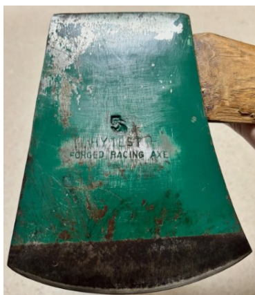
A mid-1950s green 5lb Hytest Forged Racing Axe . Cheek stamped with ‘Hytest Forged Racing Axe’ with a ‘5’ lb weight stamp. The stamps themselves are identical to those seen on the earlier Hytest Forged Racing Axes of the late 1940s - early 1950s, but are stamped on just one of the cheeks.
