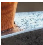
A 4½ lb Hytest Challenger axe head with a 'HAT 61' stamp on the bottom edge of the head.
