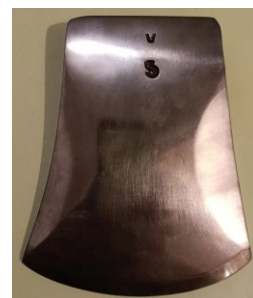
Late 1940s / early 1950s green square poll 5lb Hytest Forged Racing Axes with the 'Hytest Forged Racing Axe' stamp on the poll on one side and the '5' lb weight and a 'V' stamp on the other. The 'Hytest Forged Racing Axe' stamp was later found on the cheek rather than the poll, and then even later with both stamps (the 'Hytest Forged Racing Axe' and the weight stamps) on the cheek on the one side. (It is possible that the 'V' identifies the steel as vanadium steel alloy).
