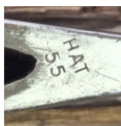
A 5 lb Hytest Forester axe head with a 'HAT 55' stamp on the bottom edge of the head.
