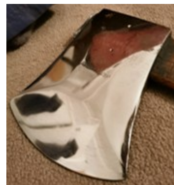
Cyclone Hytest 'felling' axes ground and hung as racing axes
